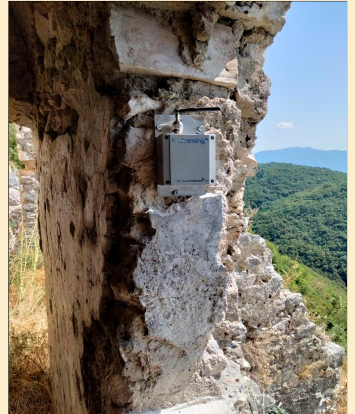
Fig. 1: Installation of a tiltmeter at the Conventillo site for monitoring structural inclination.
